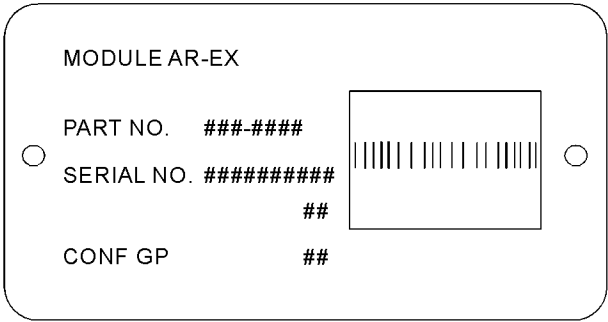
Illustration 36 g02109493 Engine aftertreatment system identification plate
