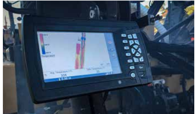
The live view display helps keep the operator informed of laydown mat temperatures.
