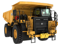
775-08 NEXT GEN (TIER 2/TIER 4/ STAGE V) 65 MT/71.5 T Decatur/Tiruvallur
