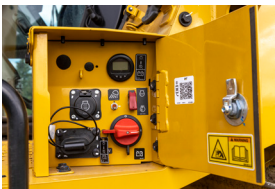
GROUND-LEVEL SERVICE CENTER
