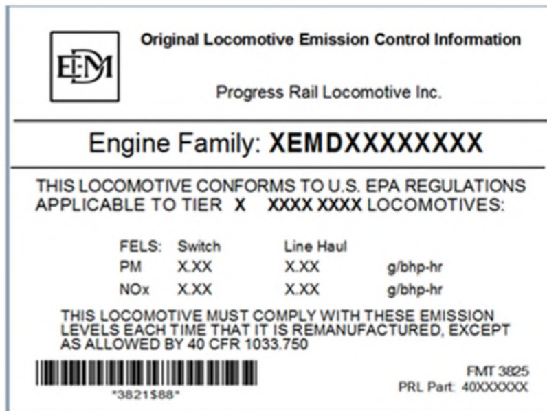
Label 2: Sample Locomotive Label. Contains “Original Locomotive Emissions Control Information” in the title.
