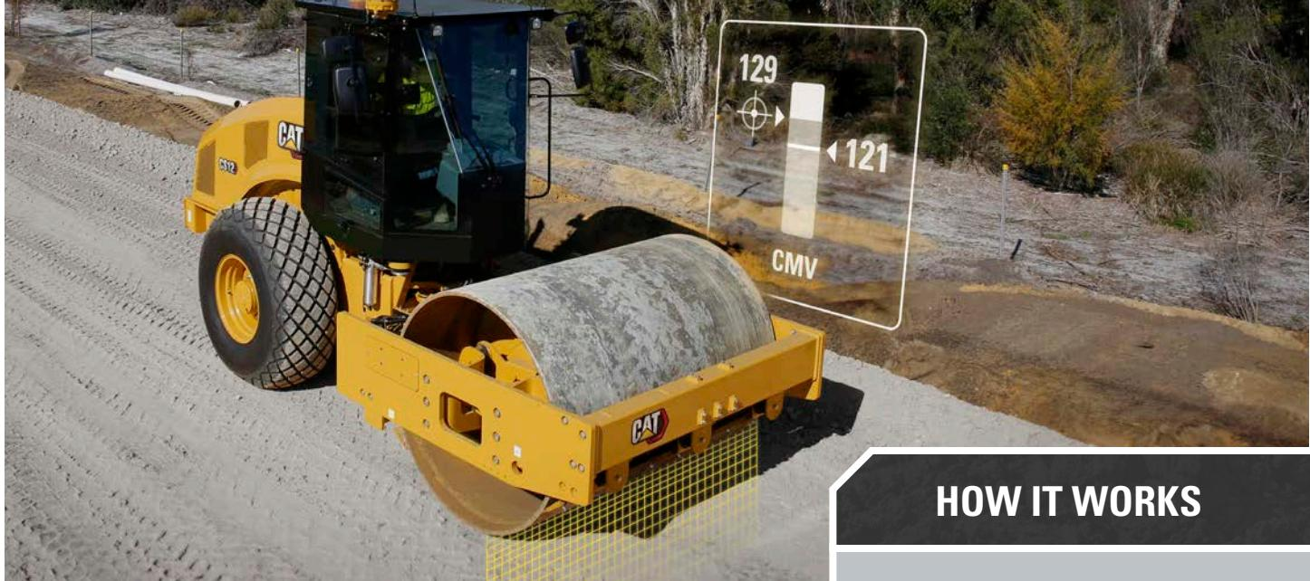
Compaction Meter Value (CMV) is an accelerometer-based technology that uses machine vibrations to measure soil stiffness during compaction. By analyzing the frequency response of the drum, CMV provides real-time data that helps operators achieve optimal compaction with confidence.
