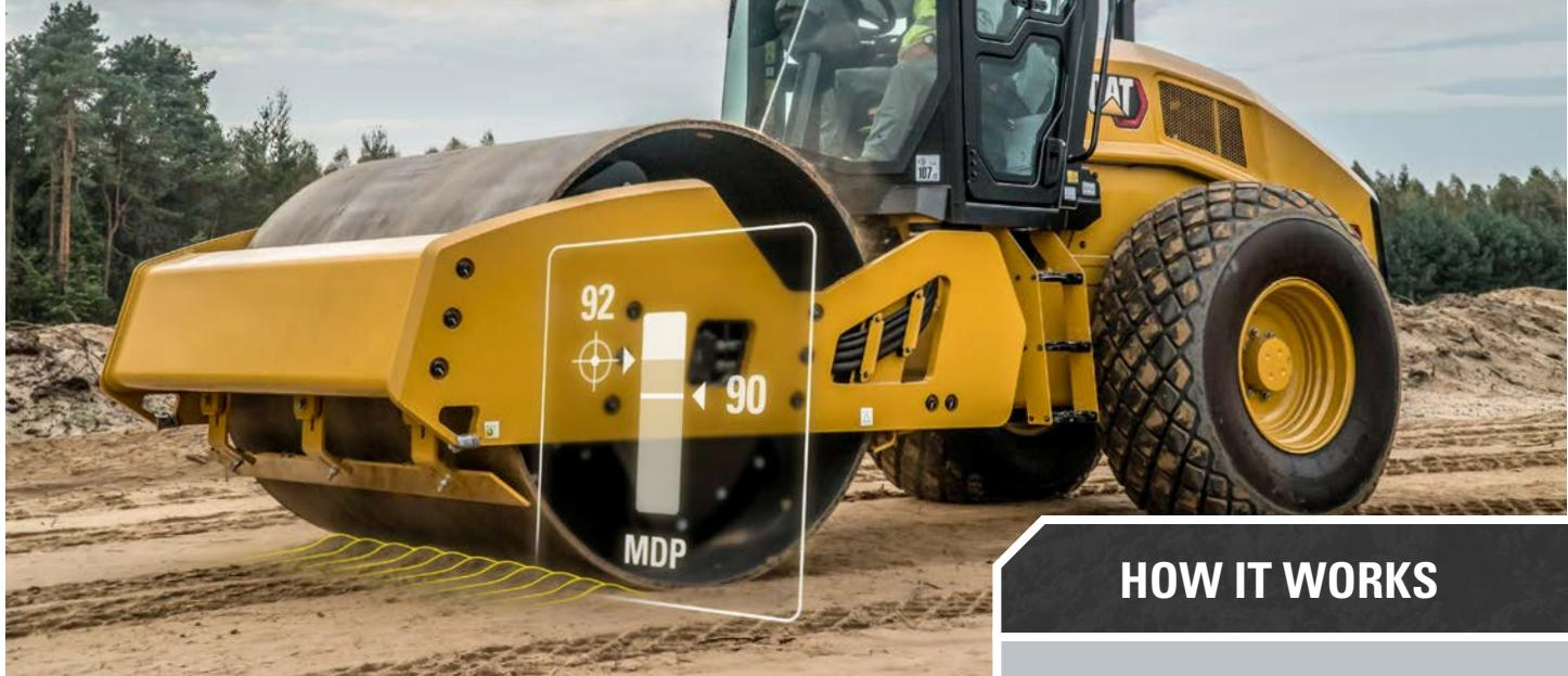
Caterpillar-exclusive Machine Drive Power (MDP) works differently than conventional methods of measurement. This energy-based technology uses sensors to measure rolling resistance and provides the operator a compaction value which is an indication of soil stiffness.
