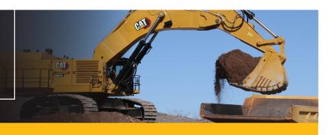
824 hp / 615 kW ENGINE OUTPUT BACKHOE: 16.1 t / 14.6 mt
