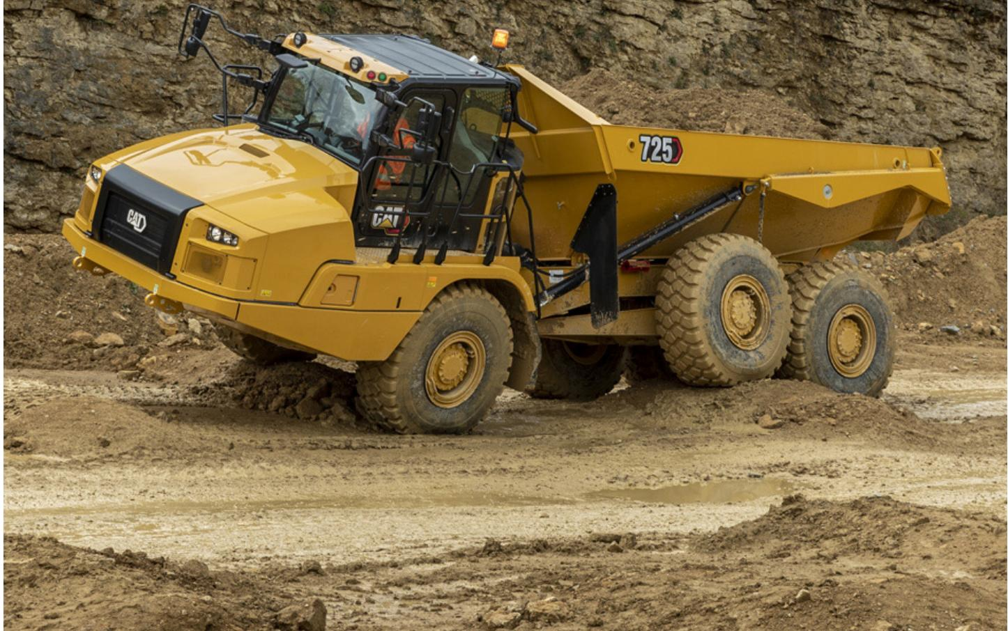
Cat® Traction Control reduces excessive tire slippage under full load conditions and improves undercarriage life. It reduces operator fatigue and increases productivity by providing a smoother reverse pass.
