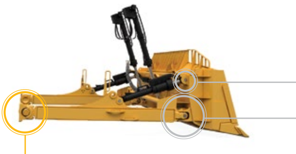
Replaceable push-arm trunnion bearing inserts
