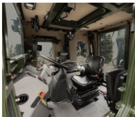
Ergonomic operator station with egress hatch in roof.
