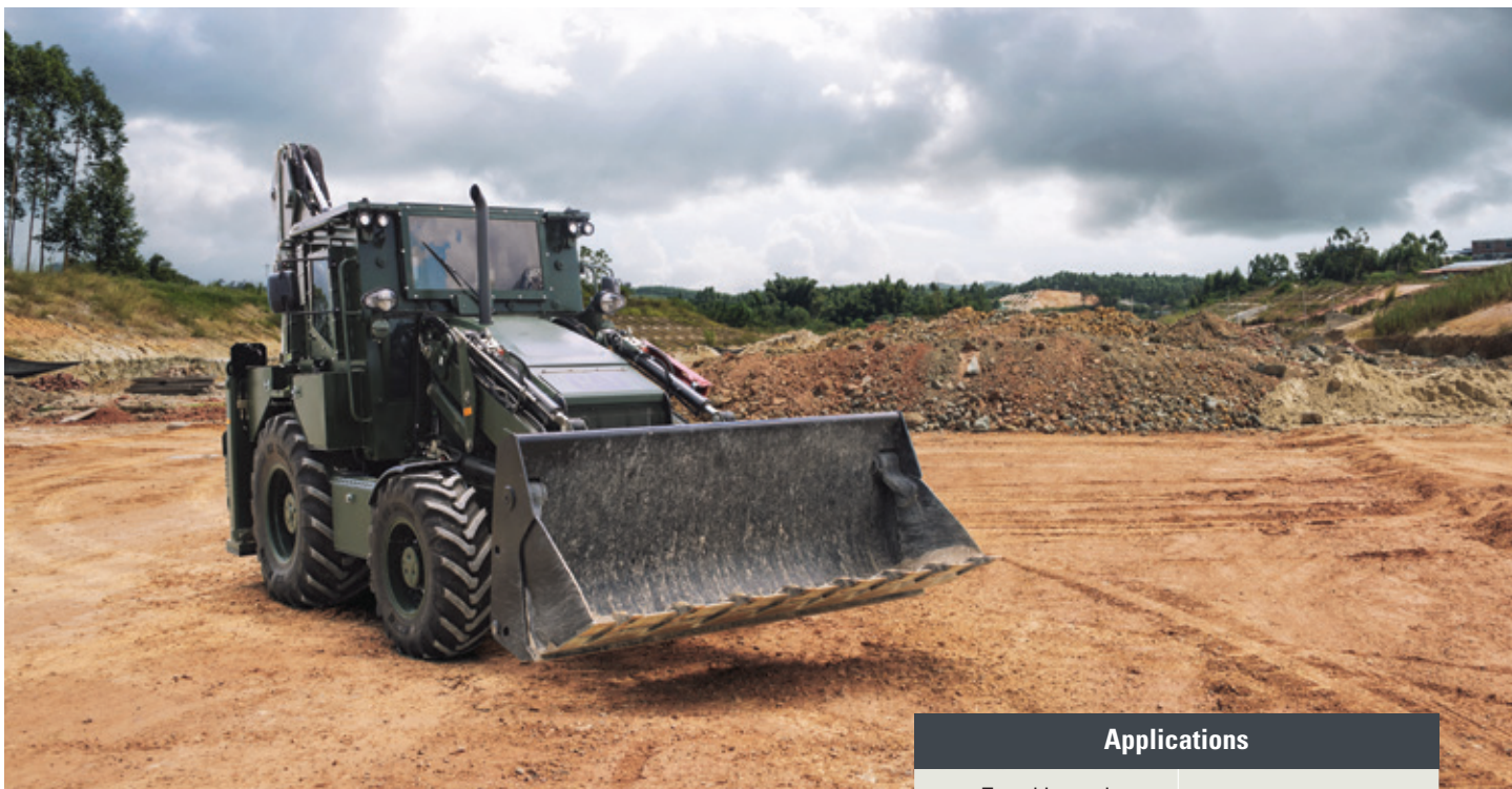
Reduced cab height for C-130 air transportability.
