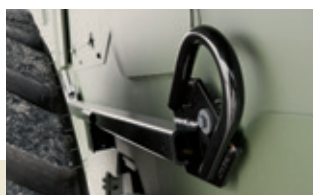
Removable bracket for C-130 air transport.
