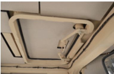
Emergency egress hatch.
