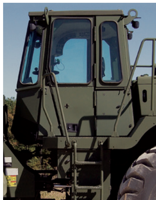
Entry ladder with self-cleaning steps and wide front and rear platforms.
