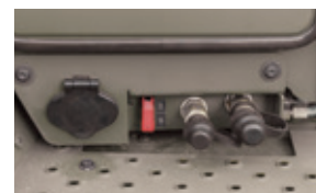
Auxiliary hydraulic hand tool circuit.
