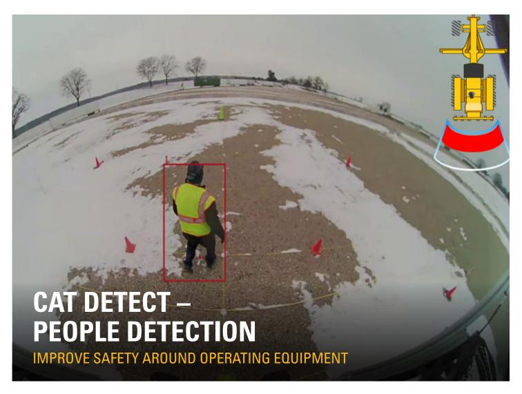
Cat Detect – People Detection is an intelligent vision camera system that can alert an operator when someone enters a machine's hazard zone.\* The system highlights people in red bounding boxes on the in-cab monitor to help operators more quickly manage potential risks.
