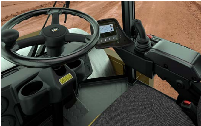
Operator environment shown with ROPS/FOPS cab and cloth seat.
