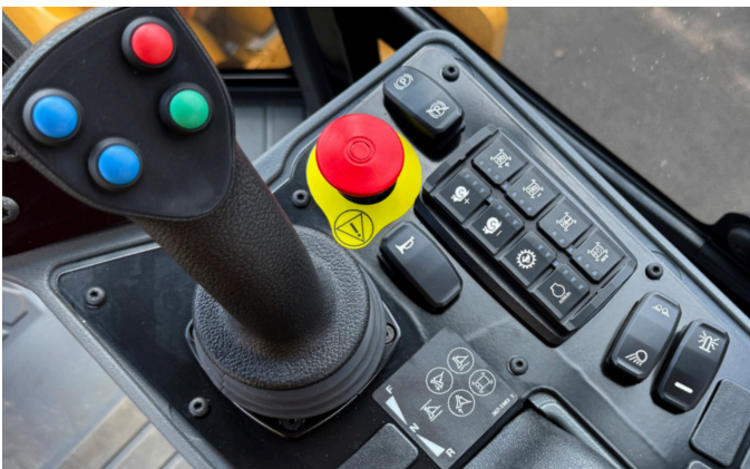
Propel lever shown for machines equipped with the optional leveling blade.
