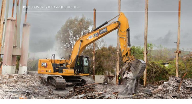
automatically stop motion when the front linkage reaches the defined boundaries, enabling operators to work with greater confidence and reduced stress.
