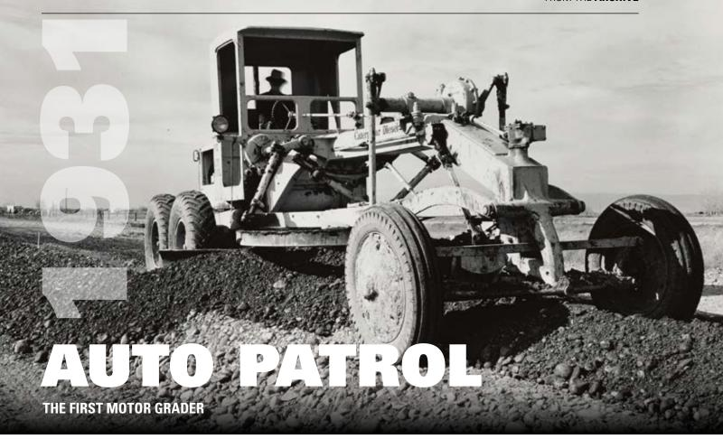
In an era when grading roads required both a tractor and a grader frame, Caterpillar developed a better way. After acquiring the Russell Grader Manufacturing Company, leaders from both companies combined their technologies in 1931, creating the Auto Patrol, the world's first motor grader.
