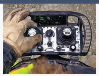
For line-of-sight operation, the Cat Command Console enables the user to work safely and comfortably outside the machine, while remaining onsite and in direct visual contact. The console provides line-of-sight operation from distances up to 437 yards away.
