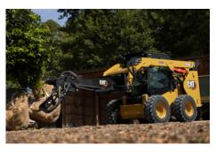
Large capacity with the ability to handle root balls ranging from 711-1321 mm (28-52 in) in size.
