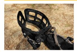
**Paddles** are shaped to wrap around the root ball without damaging the root system or tree.
