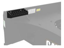
**Heavy duty bolt-on serrated step** provides secure footing for operators entering and exiting machines.
