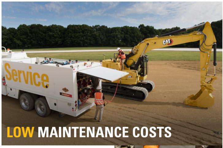
Keep your machine running longer with less hassle. Extended-life fuel, hydraulic oil, and air filters – along with the elimination of pilot and case drain filters – mean less replacements and low maintenance costs over time. Plus, a convenient ground-level engine oil check makes your daily inspections fast and safe.
