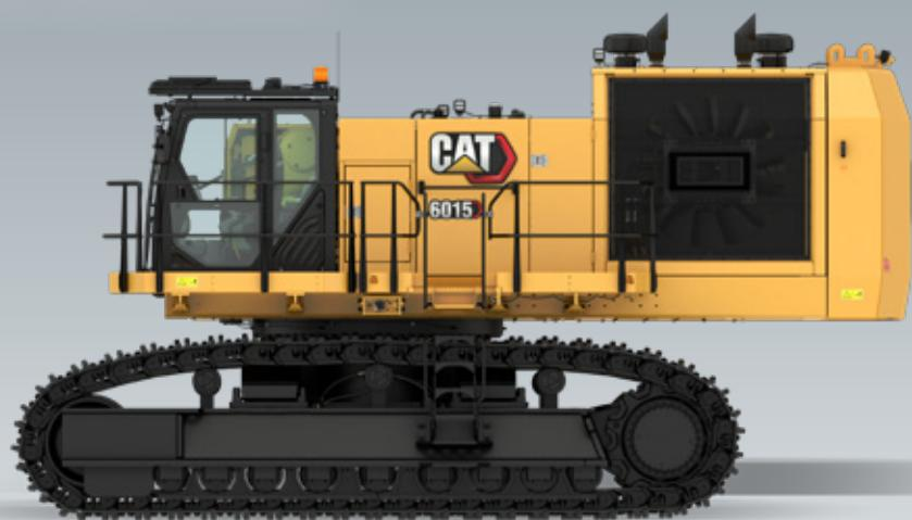
**We offer frontless mining shovels to pair with 3rd party custom attachments.** Partial mining shovels can be used for scrap, refuse, bulk material handling, dredging, demolition, specialty excavation, and forestry.
