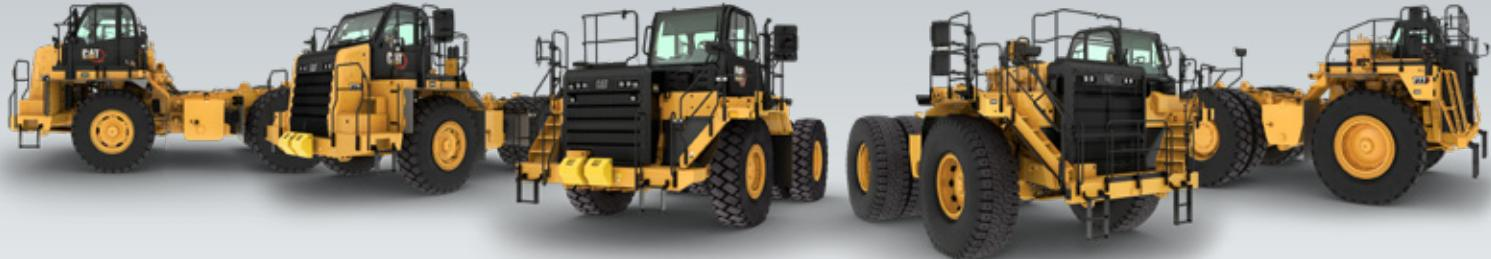
**Cat off-highway truck bare chassis options provide custom solutions for specialty applications — including water trucks, fuel / lube, and towing applications — with support from Caterpillar and the Cat dealer network.** We also offer Cat components for equipment hauling trailer arrangements and bottom dump trailers compatible with the following truck models: 775, 777, 785D.
