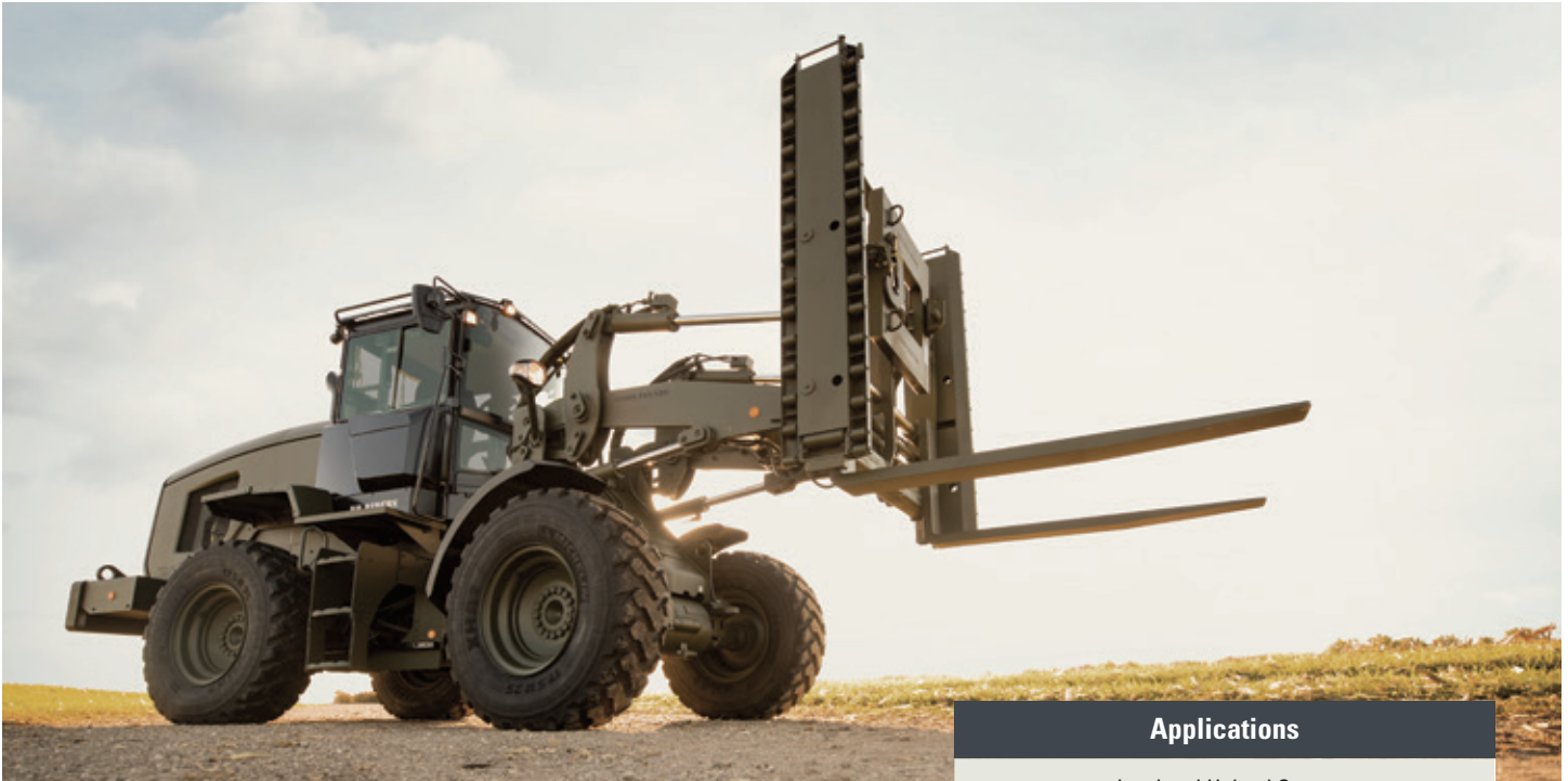
Conveyor style rollers stowed on fork carriage.
