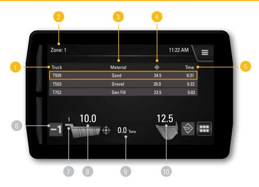
Dispatch for Loading works with Advanced Payload to provide loader operators with all the details needed to load the correct truck with the right amount of material.
