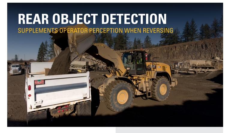
Rear Object Detection for wheel loaders is a system providing enhanced blind spot awareness. Radar provides visual and audible alerts when objects enter a safety proximity zone, while the camera allows the operator to see what's behind the machine when reversing.
