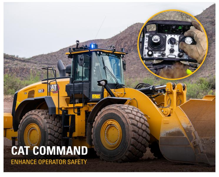
Cat Command is a sophisticated remote control system that takes operators off the machine and away from potential dangers when working with hazardous materials or in unsafe conditions. It also maintains the option to utilize other advanced control technologies, such as Cat Payload, and other machine-specific assist features.
