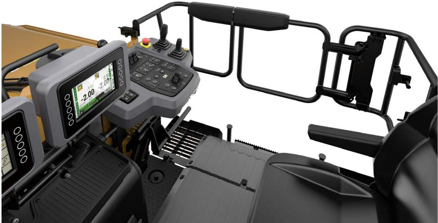
The work area can be set up for operator preference and working position. Touchscreen displays provide access to the gauge cluster, operating information, remote camera feeds, machine controls and diagnostics.
