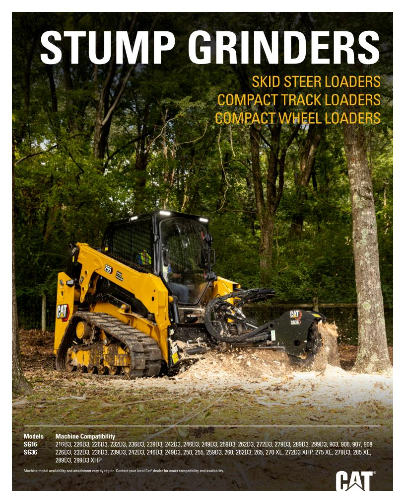
Cat® Stump Grinders are designed to economically remove stumps in residential, commercial and agricultural settings. They offer increased production over tow-behind grinders in situations where multiple stump removal is required. The right balance of cutting wheel speed and torque makes quick work of most tree varieties.
