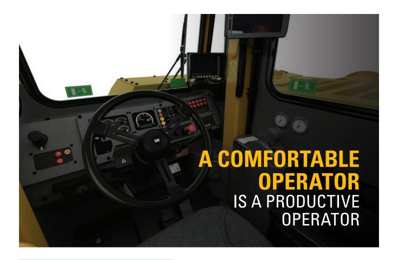
The AD45's operator station is ergonomically designed for greater control in a comfortable, productive, safe environment. Controls, levers, switches and gauges are positioned to maximize productivity and minimize operator fatigue. An ergonomic, fully adjustable suspension seat offers superior comfort for long shifts.
