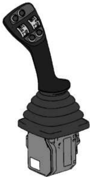
Illustration 1 g06311091 541-7470 Joystick Control As
