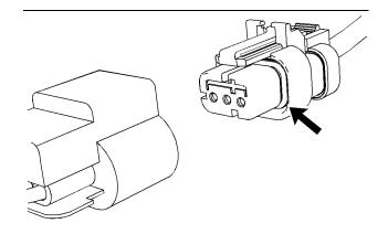
Illustration 120 g01131019 Seal for a three-pin connector (typical example)
