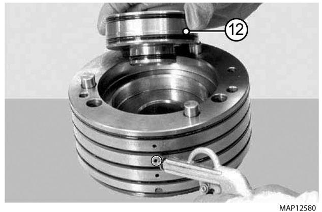
17. Applying pressure to the second hole, remove the hydraulic block piston (12).
