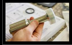
Our couplings are forged and machined from high tensile strength steel. Then they are heat treated and plated to ensure maximum durability and corrosion resistance. Salt spray testing is in accordance with ASTM B1117.
