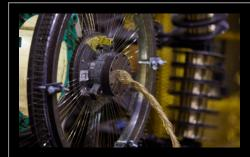
Before application, the hose is routed through a cooling chamber until it reaches a suitable temperature that prevents perforation of the hose as the high tensile strength reinforcement wire is applied.
