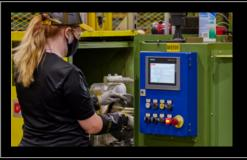
The Cat hose is carefully monitored to ensure precise inner and outer diameter measurements are maintained. This provides precise coupling retention capability.
