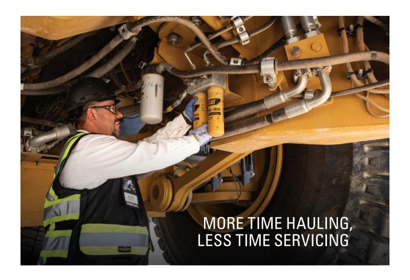
The 798 AC was designed to reduce the time you spend on regular maintenance procedures. The standard Product Link™ Elite monitoring system delivers critical health and payload information in real-time, keeping performance at optimum levels and allowing advanced troubleshooting and planning to lower maintenance costs.
