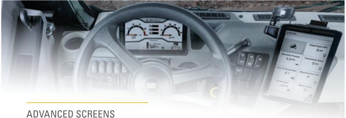
Machine data, controls and guidance information are consolidated onto two 10-inch screens to reduce the number of displays required and present the right information when needed. The screens are ideally located to enable the operator's eyes to remain forward as much as possible, reducing fatigue and improving
