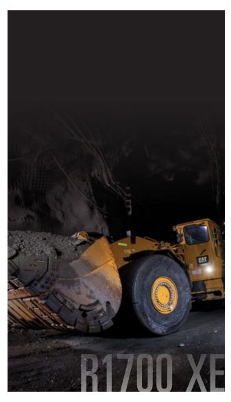
As mines dig deeper, development costs grow higher. It becomes increasingly difficult and costly to get clean and cool air. Recognizing the demand for a battery electric vehicle in deep, difficult-to-ventilate underground mines, we started with a proof-of-concept system on an R1300G in our proving ground facility. That machine was validated for more than 800 hours on a real mine site, and it demonstrated the potential of our onboard battery charging system.
