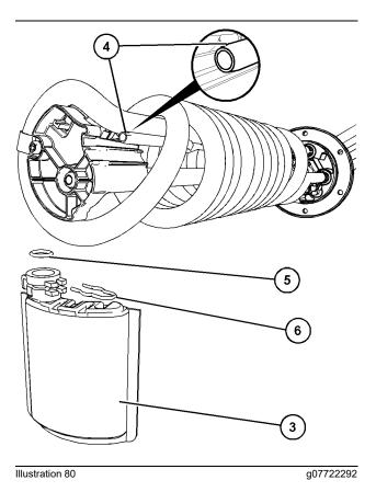
3. Pull locking clip (6) outwards and remove the DEF
