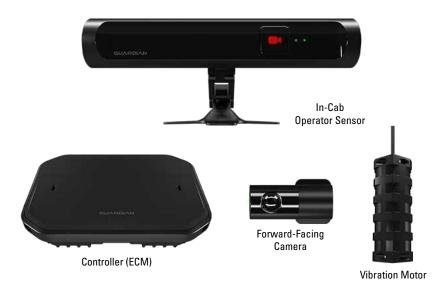
The Cat Detect DSS in-cab hardware is a comprehensive system comprising an operator-facing sensor that detects facial and eye changes, an electronic control module (ECM), a vibration motor, and a forward-facing camera\* that provides video of events that occur in front of the machine.
