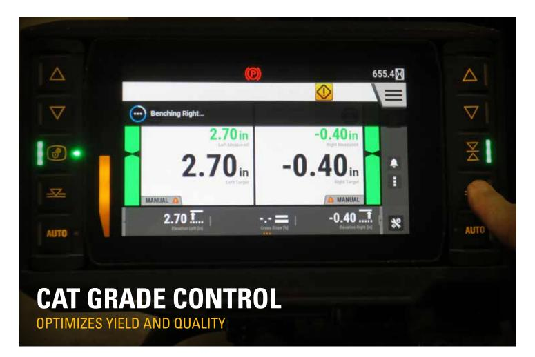
The Cat Grade Control option helps deliver smoother surfaces and control mat thickness for increased performance, lower operating costs, and higher profitability. Text-based user-friendly displays, accurate control, and great reliability can help ensure quality targets are being met.
