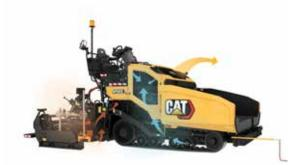
The standard ventilation system draws air from the conveyor tunnel as well as the auger chamber and redirects it away from the operator for a more comfortable working environment.
