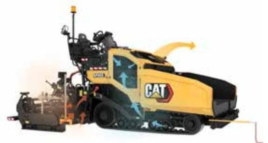
**The standard ventilation system draws air from the conveyor tunnel as well as the auger chamber and redirects it away from the operator for a more comfortable working environment.**
