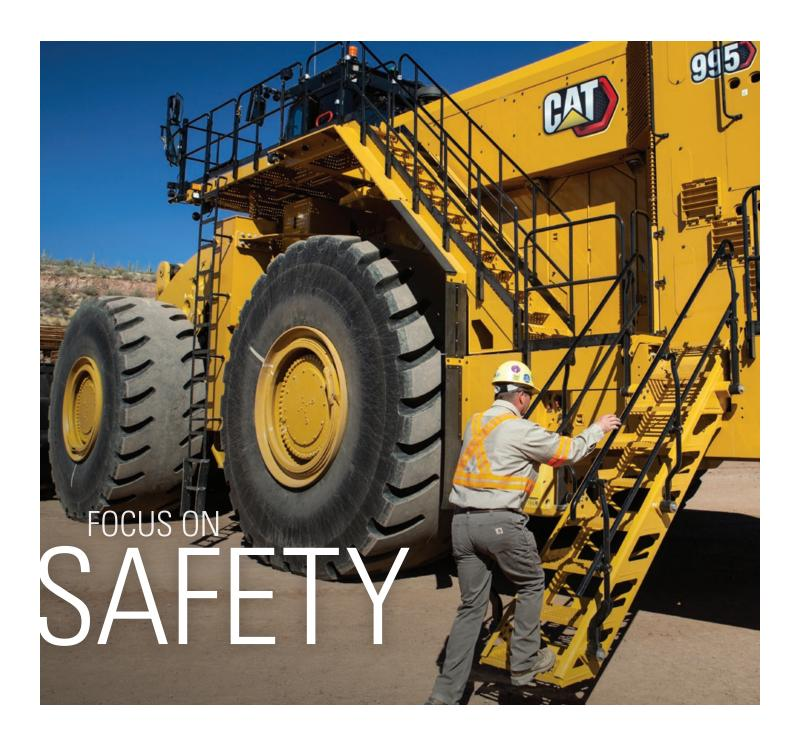
From slip-resistant surfaces and guard rails to state-of-the-art object detection technologies, the 995 is infused with features to help both operators and service personnel feel safe and confident on the job. We've improved access and egress, maximized visibility and made it possible to perform more service from the ground.
