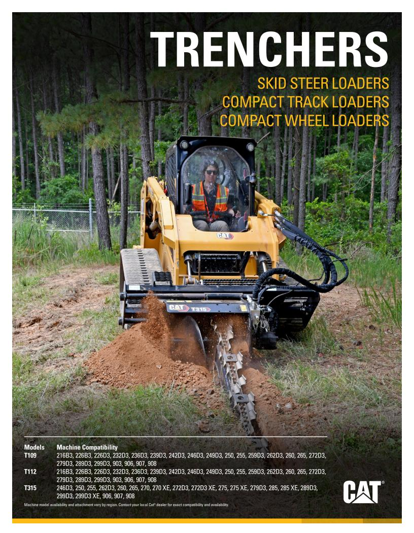
Cat® Trenchers are designed for cutting narrow straight trenches in the soil prior to laying electrical, telephone and cable lines, or water and gas pipe. Trenchers are ideal for residential, commercial, agricultural, building construction, lawn care and golf course maintenance.
