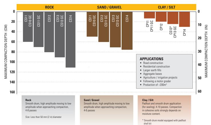
Assumes density specification is 95% of Standard Proctor and can vary substantially due to different soil conditions.
