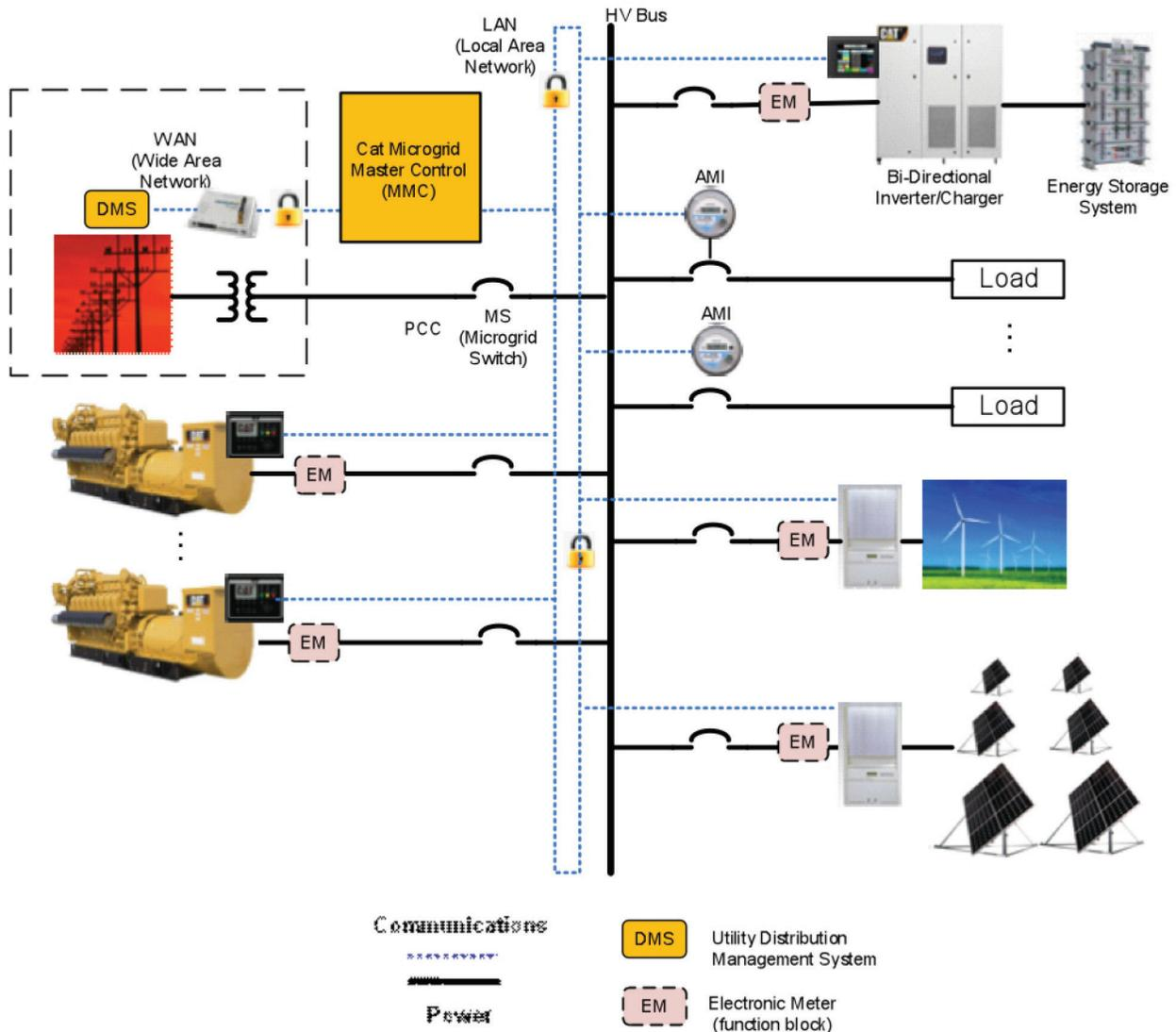
Figure 1: Typical single-line diagram of a hybrid microgrid
