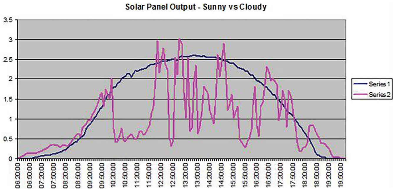
Figure 5. Solar panel output: sunny vs. cloudy
