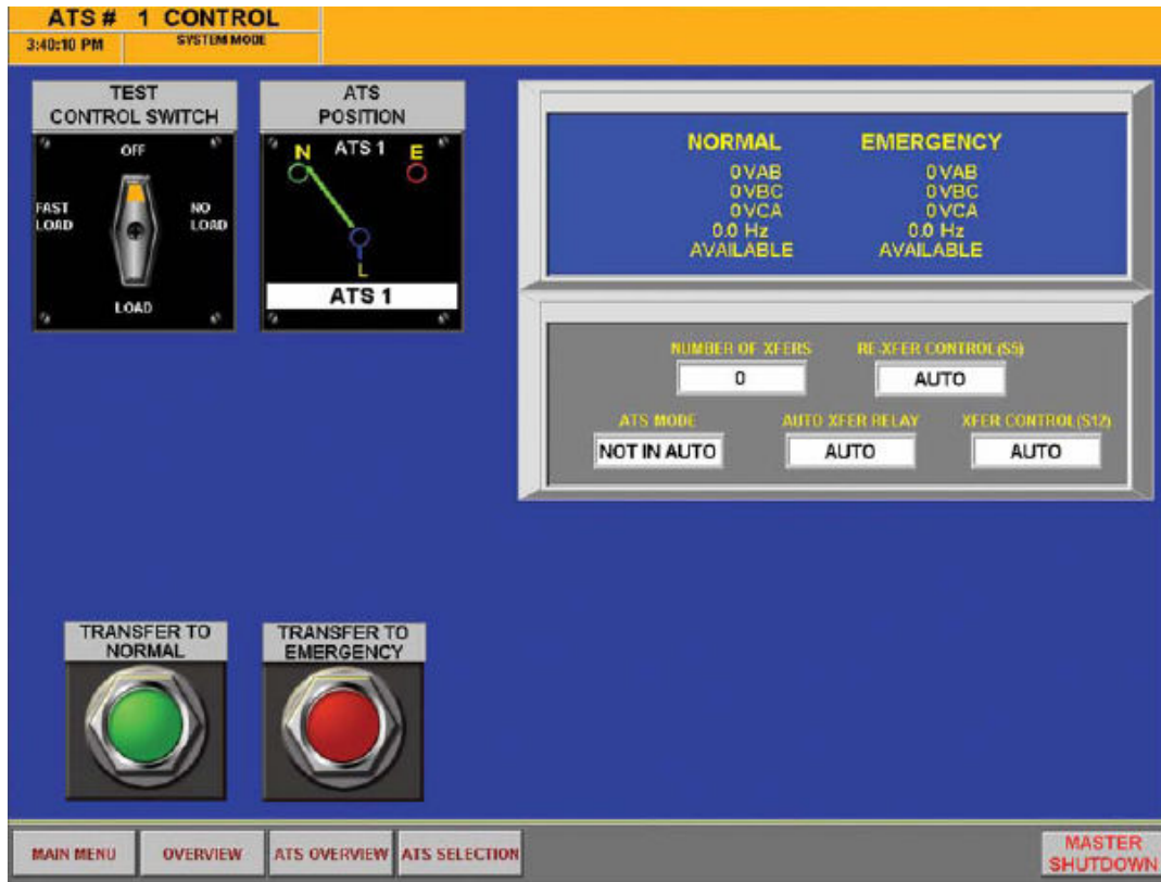
Figure 10 – ATS Remote Monitoring Software Screens
