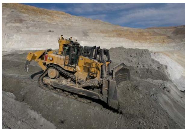
Figure 6. The D10 proved to be 3 – 7% more productive than the D10T2 in all tests, and its stator clutch torque divider improved efficiency.
