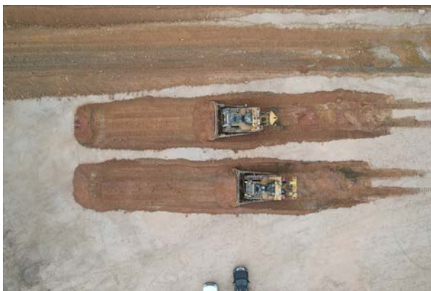
Figure 3. One test included two sets of six slots with a level test area, flat loading and carry segments, and the fill producing a 5% uphill grade.
