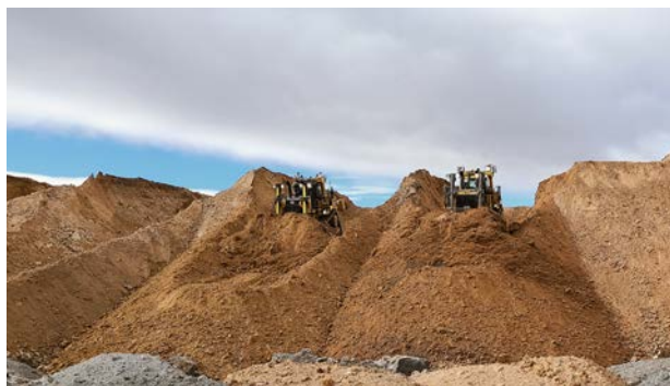
Figure 4. Dozer speed tests proved the D10 was 5% faster in reverse, and its optimised forward gear offered 5% more cycles per hour than the D10T2.
