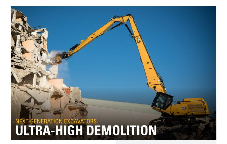
Cat ultra-high demolition excavators are the optimum solution for demolishing structures up to nine stories high using a range of Cat demolition attachments, including multiprocessors, grapples, shears, and hydraulic hammers with the retrofit boom.
