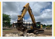
Auxiliary hydraulics give you the versatility to use a wide range of Cat demolition attachments, including hammers, shears, pulverizers, grapples, and more. The counterweight ensures stability with even the heaviest attachments.
