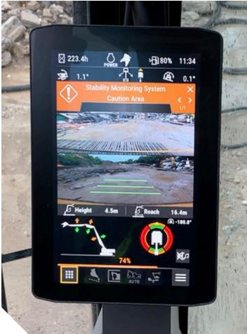
The Cat stability monitoring system on machines with UHD fronts keeps you continuously aware of attachment position within the safe working range. The system monitors the front position and swing angle. Audible and visual indicators warn the operator when nearing the stability limit.
