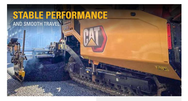
Steel track models provide many of the same great features utilized on the Mobil-Trac versions with slightly less travel speeds. This stable design utilizes an auto-tensioning system for excellent tractive performance while keeping wear at a minimum.
