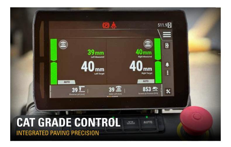
The Cat Grade Control option helps deliver smoother surfaces and better control of mat thickness for increased performance, lower operating costs, and higher profitability. Text-based user-friendly displays, accurate control, and greater reliability can help ensure quality targets are being met.
