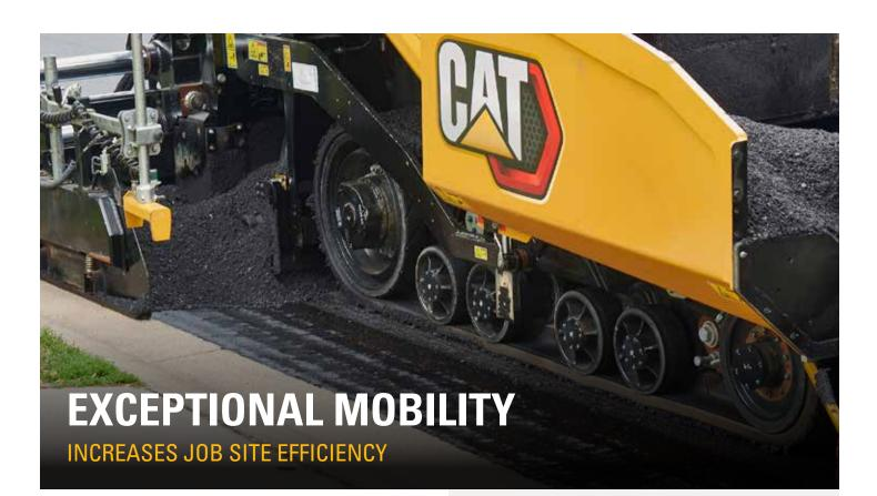
Mobility is one of the keys to job site efficiency, maneuvering in confined areas, backing up to curbs and repositioning at the starting point are real advantages of the Cat Mobil-Trac<sup>™</sup> system.
