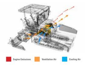
The engine emissions are directed out over the hopper. When equipped with the optional ventilation system, air from the conveyor tunnel and auger chamber follows a similar path and is redirected away from the operator for a more comfortable working environment.
