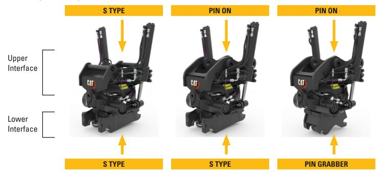
The S Type lower interfaces use industry standard sized S couplers, which can pick up S Type attachments. The S Type lower interface is compatible with the optional integrated grapple. The pin grabber lower interface uses the standard Dual Lock pin grabber coupler. It can pick up any attachment with the pin on interface. The pin grabber lower interface is not compatible with optional integrated grapple.
