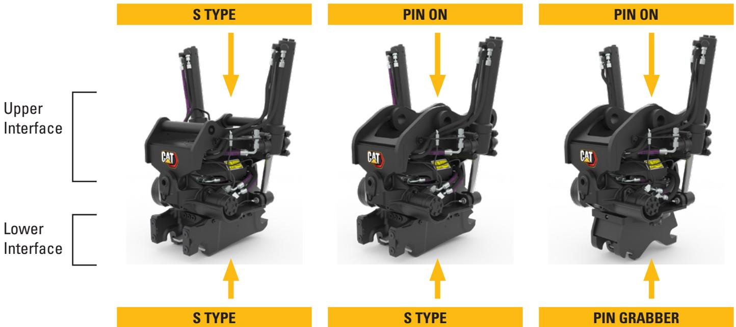
The S Type lower interfaces use industry standard sized S couplers, which can pick up S Type attachments. The S Type lower interface is compatible with the optional integrated grapple. The pin grabber lower interface uses the standard Dual Lock pin grabber coupler. It can pick up any attachment with the pin on interface. The pin grabber lower interface is not compatible with optional integrated grapple.
