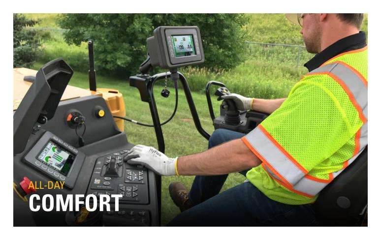
The work area can be set up for operator preference and working position. Touchscreen displays provide access to the gauge cluster, operating information, remote camera feeds, machine controls and diagnostics.
