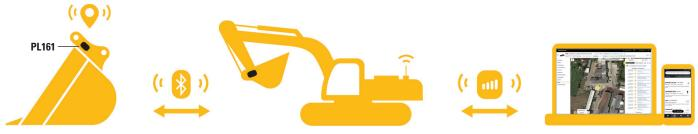
PL161 sends a signal to the Bluetooth receiver or PL542 on the machine.
