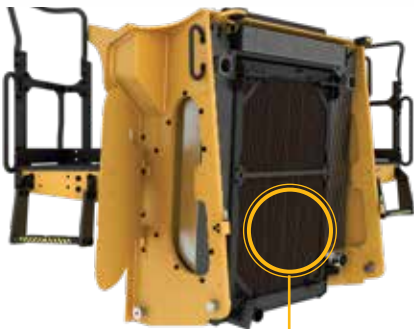
Single plane cooling system reduces heat load for longer component life
