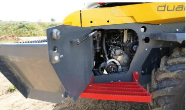
Additionally, the Perkins engine used is equipped with an auto stop function which switches off the engine if the machine is not used for a pre-set time. This time can be set by the user and can also be turned off.
